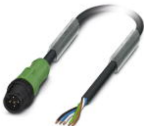
Sensor/Actuator cable, 5-position, PUR halogen-free, Black-gray RAL 7021, Plug straight M12, A-coded, on Free cable end, Cable length: 1.5 m, with plastic knurl
